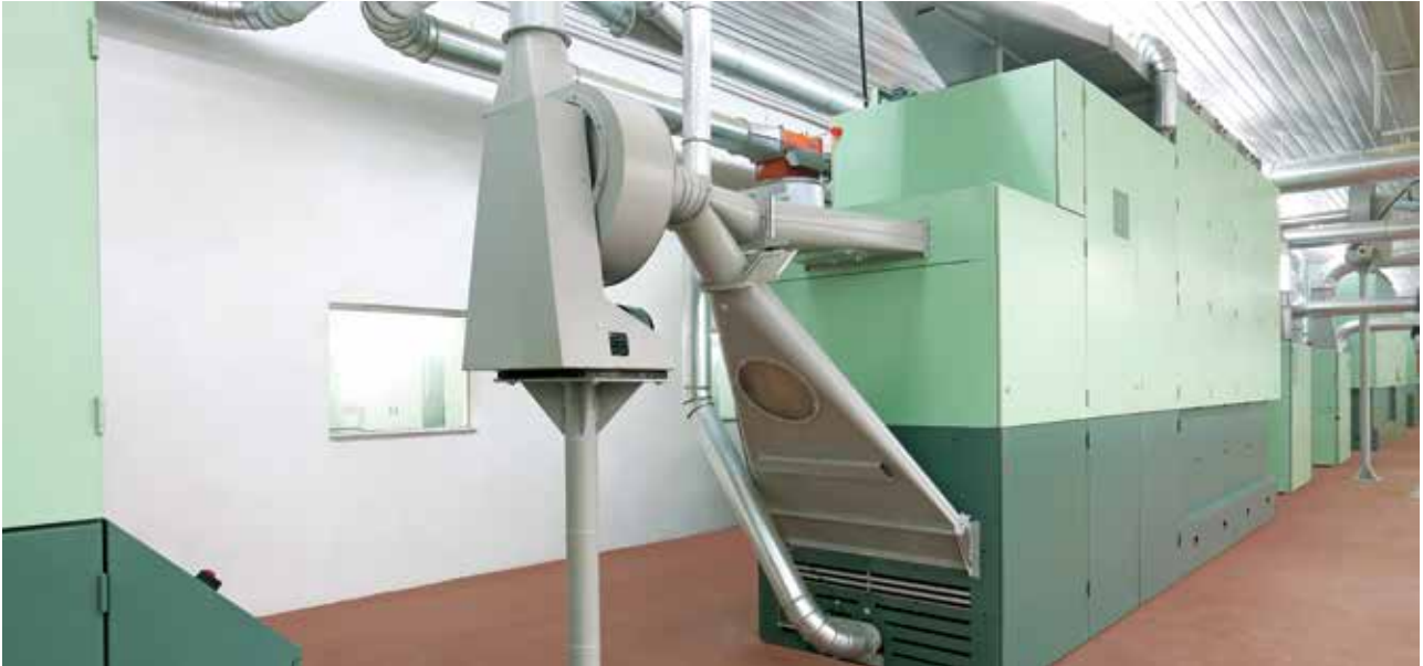
Fig. 5 Optimal cleaning with the B 72 R UNImix, seen here with the module to bypass the cleaning positions
