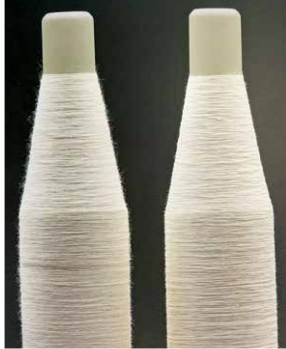
Comparison between standard ring yarn and Mac3000 compact yarn
